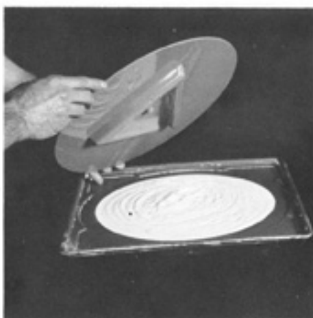
Seat quick-release into back of mold.
