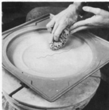
Center mold on wheel (Giffin Grip or clay chuck is helpful) & sponge slab to desired contour.
