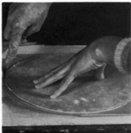
Roll out a clay slab. Trim to fit & place in mold.
