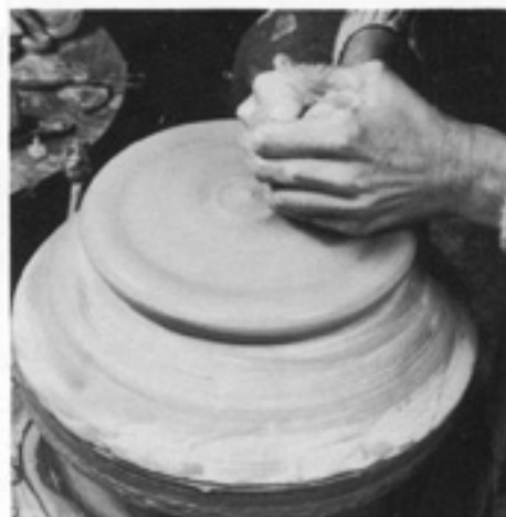
Dampen bat evenly. Apply a measured clay paddy or slab onto bat.
